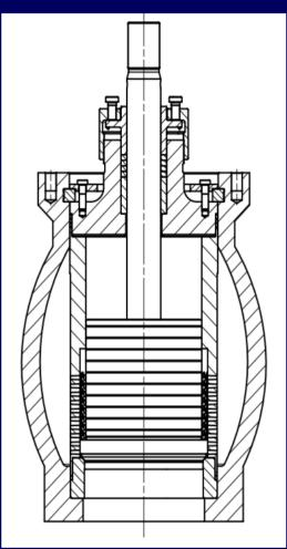
Carter Process Control GmbH has been working with clients to reduce their maintenance and downtime by upgrading the Bypass Valves of CCI/BTG VLB & VLR valves to a quick change removable seat replacing the original welded in design.
