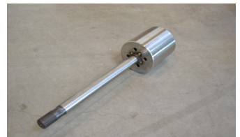
A simple drilled hole cage we were asked to manufacture for a UK Power Station
